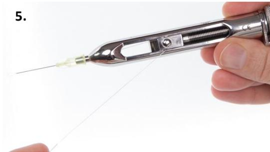
5. With light pull on the insertion aid (15), the wire (14) is to be threaded through the gap between the locking nut (7) and slide (2) and then to be wound about 90 ° around the lead screw (6).
